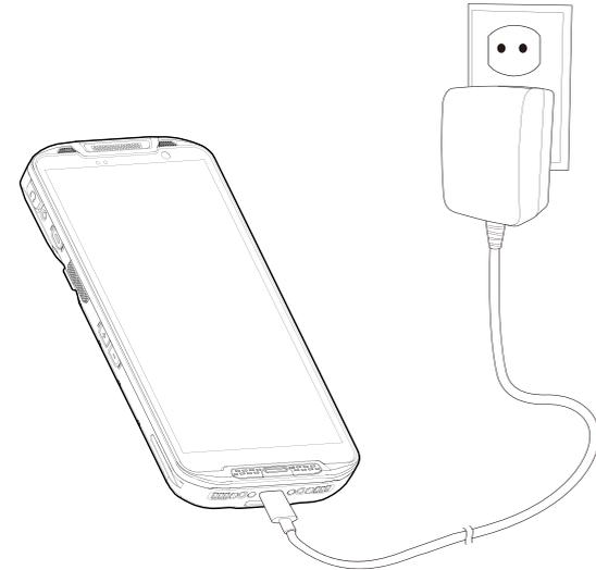
1. Assemble the AC plug and charger, and rotate the plug clockwise to engage firmly.
