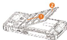
4. Insert battery cover, top first and press it in the order named on the picture. Then press down on battery at the center again.
