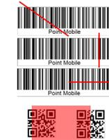
If you aim the barcode wrong direction or aim point is too tilted to scan only the part of the barcode, you can't read the barcode.
